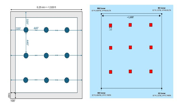
Schematic drawings showing example of the patch reef (n=9) proposed design. The blue stars (n=9) represent a single patch reef, and the arrows show their proposed placement relative to the proposed permit boundaries and distance to other patch reefs within the site. Less than 1 acre of total seafloor will contain artificial reef materials at this site.
